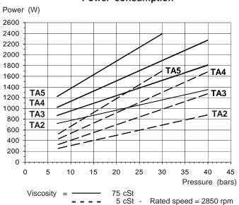
Data shown are for new pumps, with no allowance for wear.
